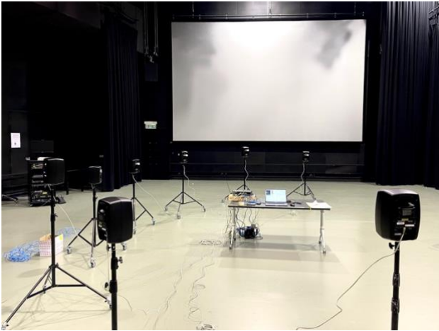
Figure 1. SoundLab: circle of twelve loudspeakers at floor level.
