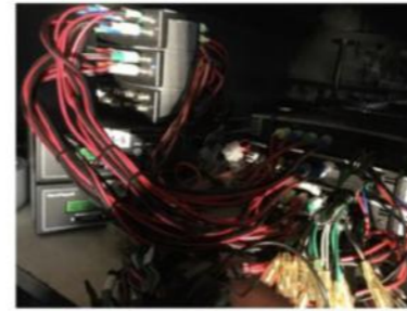
The equipment platform conceals playback devices, pre-amplifiers, amplifiers, and cables
