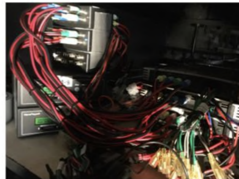
The equipment platform conceals playback devices, pre-amplifiers, amplifiers, and cables
